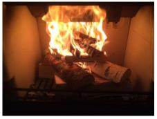
Allow the fuel to reach a steady burn and usually the initial fuel can be left to burn down to charcoal without much further attention. Build the fire up carefully by adding a couple of small
