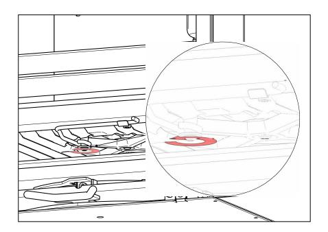
**9.6 Removing Flue Spigot Collar.** Unscrew and remove 4 x M6 securing screws from inside the firebox and remove spigot collar. When re-assembling either use a suitable fireproof gasket or fire cement.
