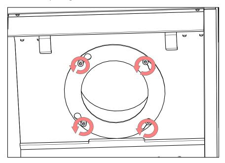
**9.7 Removing and re-fitting Trim.** 1. Remove Trim Top plate and stove door as described earlier. 2. Remove 2 x upper trim securing screws and 2 x lower trim securing screws and lift trim away. Re-fitting is a reverse of removal, noting that the trim fits behind the door hinges and door latch brackets and so may need to be slid in from above or one side fitted before the other and then slid down behind the lower hinge and latch bracket.
