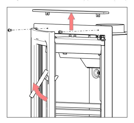
**9.2 Removing Door.** Remove the stove door by opening to approximately 30 degrees and lifting away to disengage the hinge pins. It is not necessary to remove the door to clean or remove items from inside the firebox.
