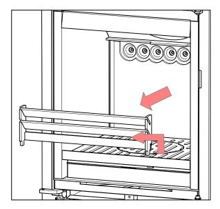
**9.5 Removing Grate components.** 1. Unscrew the operating rod from the underside of the centre rotating grate section using a 10mm AF spanner. 3. Lift out the two grate sections. 4. The operating rod can then be removed by unscrewing the support bracket(s).
