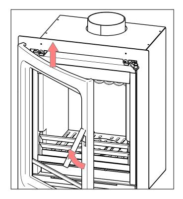
9.3 Removal of or Inspection Above Baffle Plate. First lift upwards at the front and at the same time sliding the rear forwards off the back baffle support bracket. 2. Next lower the rear edge into the firebox and allow the front of the baffle to slide off the front baffle support brackets. 3. Finally rotate the baffle out of the firebox.
