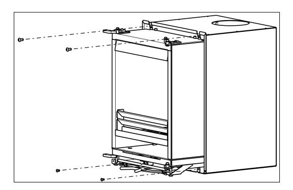
**9.9 Door Hinge Adjustment.** Door alignment may be adjusted by slackening the door hinge securing screws and re-positioning the hinge to suit. This will adjust the horizontal alignment. For front-back alignment carefully adjust the hinges mounted on the stove body. Check the door seals with a paper strip all around after any adjustment to prove they are still sealing correctly.
