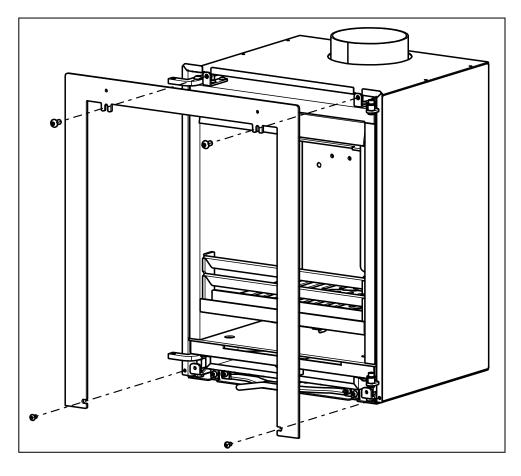
9.8 Removing Inner Firebox from Outer Casing. 1. Unscrew 2 x M6 screws securing lower outer casing to outside air box. 2. Unscrew and remove 4 x M6 screws from both left and right upper casing brackets (if not already removed for trim removal). The inner firebox can now be slid out from the outer. A lever may be needed as the components may be a tight fit. Re-assembly is the reverse of removal.
