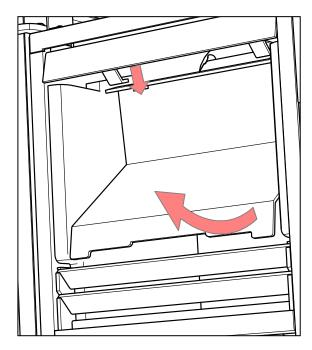
9.4 Removing Firebox Liners and Fuel Retainer Assembly. 1. First slide the front edges of the left and right firebox liners inwards at the front until they disengage from the rear liner. Then tilt them slightly and remove from the firebox – NOTE: Ensure that the rear firebox liner does not fall forwards and break! 2. Remove the rear firebox liner being very careful not to damage the profiling at the top which is delicate. 3. Remove the fuel retainer assembly by lifting up out of its slots.
