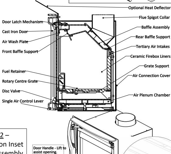
Fig 2 – **Purevision Inset** Stove Assembly and controls. 5kW model shown.
