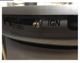
inwards and downwards into the slot until it latches fully into the **CLOSED** position allows the baffle flap to remain in the closed position permanently during all operation. This is useful where flue draw is very good even when the flue is cold.
