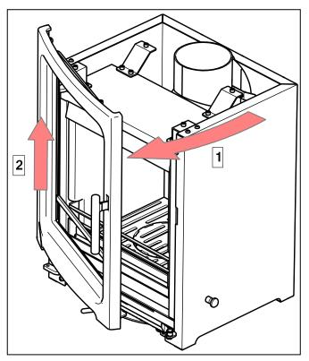
**9.2 Removing Door.** Remove the stove door by opening to approximately 30 degrees and lifting away to disengage the hinge pins. It is not necessary to remove the door to clean or remove items from inside the firebox.
