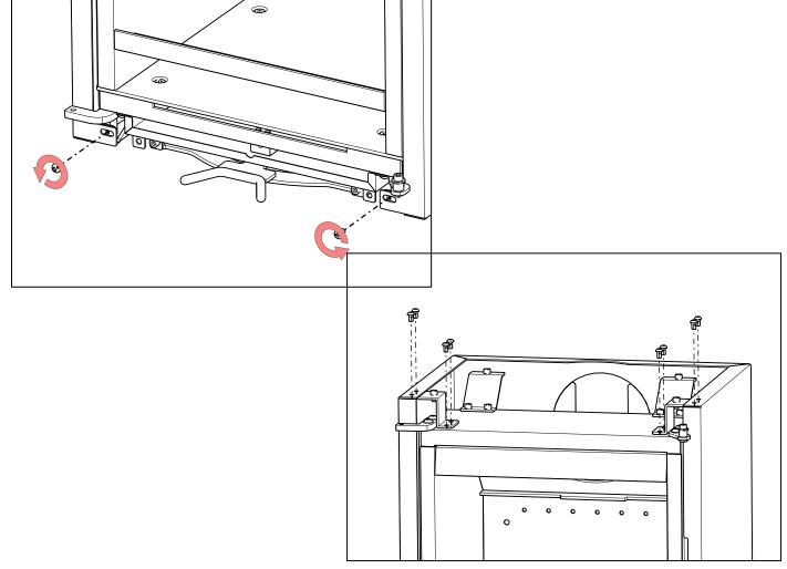
**9.8 Door Hinge Adjustment.** Door alignment may be adjusted by slackening the door hinge securing screws and re-positioning the hinge to suit. This will adjust the horizontal alignment. For front-back alignment carefully adjust the hinges mounted on the stove body. Check the door seals with a paper strip all around after any adjustment to prove they are still sealing correctly.
