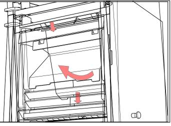
9.4 Removing Firebox Liners and Fuel Retainer Assembly. 1. First slide the front edges of the left and right firebox liners inwards at the front until they disengage from the rear liner. Then tilt them slightly and remove from the firebox – NOTE: Ensure that the rear firebox liner does not fall forwards and break! 2. Remove the rear firebox liner being very careful not to damage the profiling at the top which is delicate. 3. Remove the fuel retainer assembly by lifting up out of its slots.
