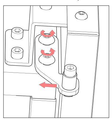
screws slightly. Now tap the end of the bracket towards the centre of the stove. This will increase engagement with the door latch forks. Now retighten the bracket fixing screws.
