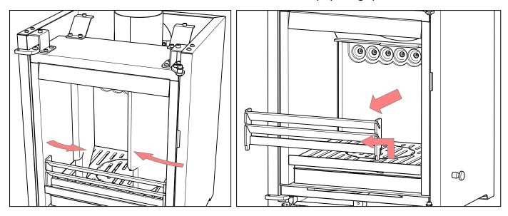
**9.5 Removing Grate components.** 1. Remove the riddling/shaker knob by unscrewing from the operating rod. 2. Unscrew the operating rod from the underside of the centre rotating grate section using a 10mm AF spanner. 3. Lift out the two grate sections and the operating rod.
