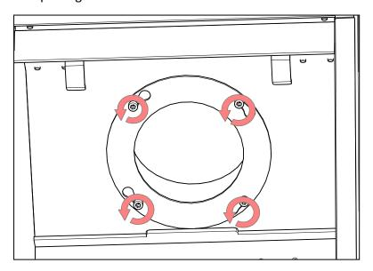
**9.7 Removing Outer Casing.** 1. Unscrew 2 x M6 screws securing lower casing to stove legs. 2. Unscrew and remove 4 x M4 screws from both left and right upper casing brackets. Remove the brackets from the firebox itself to allow removal of the casing as easily as possible.
