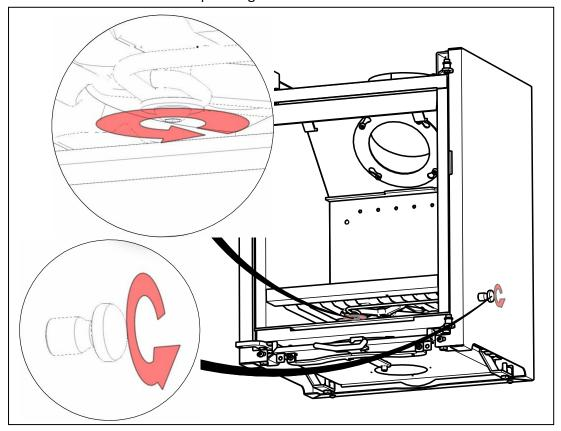
**9.6 Removing Flue Spigot Collar.** Unscrew 4 x M6 securing screws from inside the firebox and remove spigot collar. When re-assembling either use a suitable fireproof gasket or fire cement.
