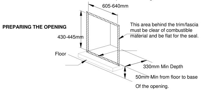
The front face and the base of the fire opening must be flat to ensure that a good seal is formed between the rear and base of the appliance and the chimney to avoid any reduction of natural draught.
