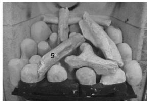
Place driftwood SHAPE No. 9 in position as shown. The recess in the base should locate over shape no.6 and the short leg should be located behind the LH side pebble. The arrow, marked on the base, should point towards the left hand side of the appliance.
