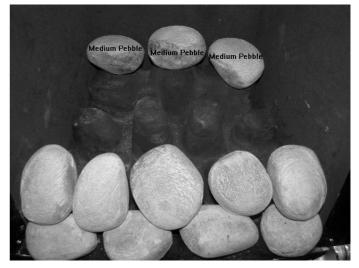
Place two heart shaped pebbles as shown on the second row of pebbles. Rest them carefully on the side liners and base matrix touching the first row laid earlier.
