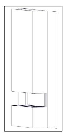
Using a 70mm core drill bit. Cut out four holes 2 left hand and right hand in the top section of the false chimney construction. The bottom hole should be positioned 265mm from the top return edge of the fascia. The top holes should be positioned 150mm down from the top edge of the false chimney breast.
