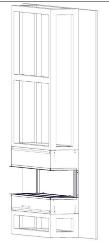
• Using suitable board and fixing, cover both side and front sections of the false chimney.
