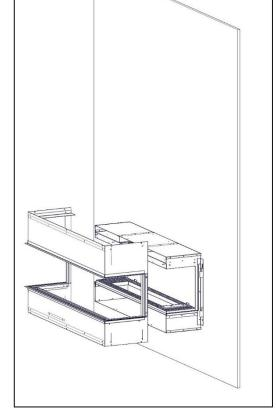
• Place a further piece of 10mm heat resistant board 956mm x 258mm within the false chimney fascia.
