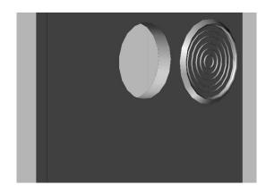
Connect and insert battery holder within the front section of frame assembly. Finally locate the inlet cover within the frame assembly.
