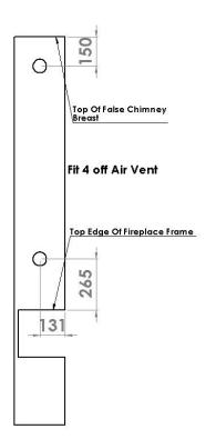
• Fit the four off 70mm diameter circular soffit vents provided with the appliance.
