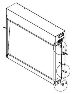
5.5cPut the fire box onto the wall bracket and then fix with two fixing screws of the wall mount brackets on the top of the fire box. Remove the front glass and arrange the fuel bed as described in 5.4c and 5.4d.
