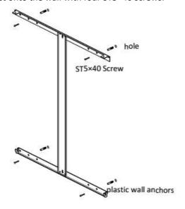
Note: For 890Eand 1500E, mark and drill four holes on the wall using this kind of wall bracket as a template and Fix the wall mount bracket onto the wall with ST5\*40 screws.
