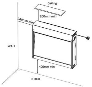
5.5aFor 780E, carefully, mark and drill four holes on the wall using the wall bracket as a template and push in the four plastic wall anchors. Fix the wall mount bracket onto the wall with four ST5\*40 screws.
