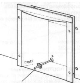
BLIND GROMMET (SUPPLIED ASSEMBLED IN INLET PIPE ENTRANCE HOLE).
