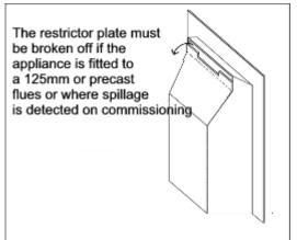
A pre-cast flue conforming to the requirements of BS 1289 part 1 & 2 A suitable fire resisting fire surround will be required, spaced out to the correct thickness, between the face of the flue blocks and the rear of the appliance frame. **IMPORTANT:**- the flue restrictor plate must not be fitted when the appliance is installed in this type of flue.
