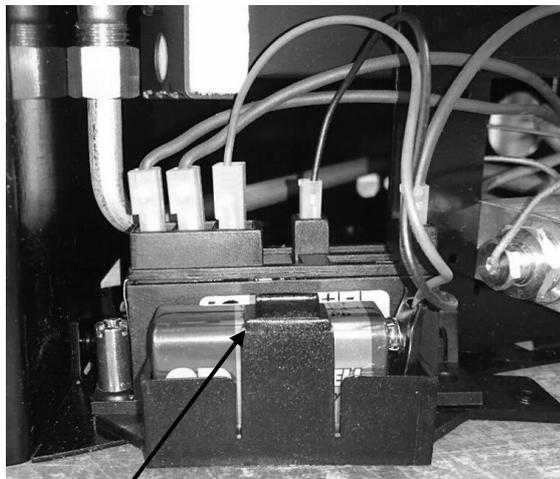
Ensure battery is located properly so this hook hold the battery in place
