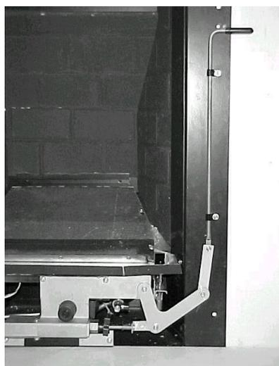
Connect the link lever to the stud at the end of the slide control lever and replace the nylock nut. **IMPORTANT TURN THE NUT UNTIL IT JUST TIGHTENS AND THEN TURN IT BACK A HALF TURN.** Check the operation on the lever and mechanism ensure that the lever springs back to the low position when it is released after pushing down.
