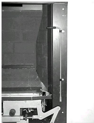
Flip the slide control lever round so that the rubber-capped end is protruding out to the right as shown in the left-hand picture. Check that it slides freely up and down in the nylon slide guides. Remove the nylock nut with a 7mm A/F spanner as shown.
