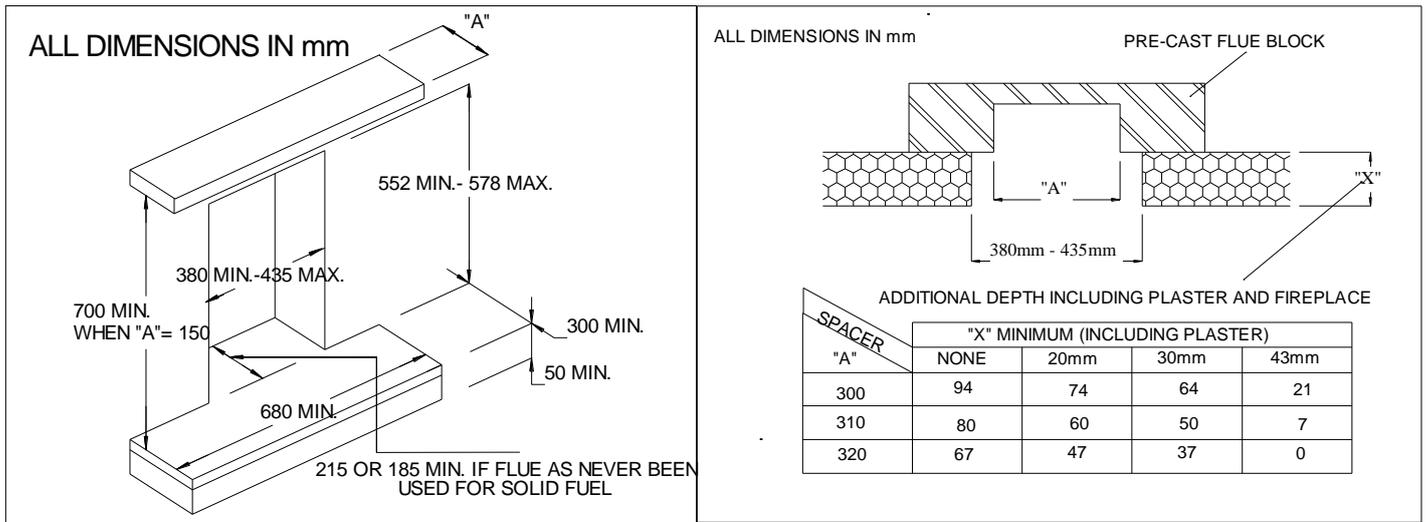
**NOTE :- LOW LINTEL OPENING HEIGHT IS REDUCED TO 500mm – 526mm.**
