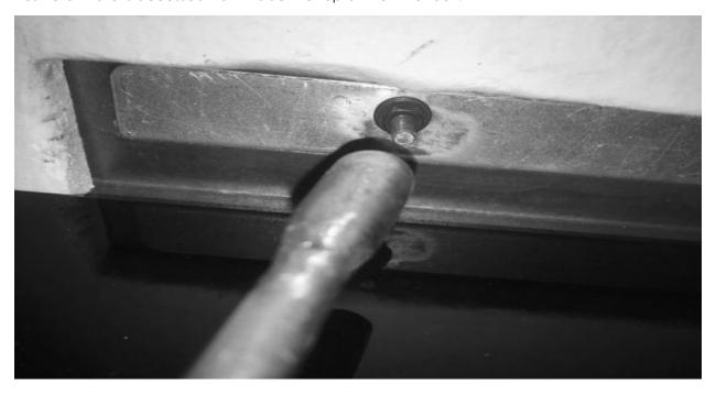
Undo the two M4 nuts, the Restrictor Plate should fall away as shown.
