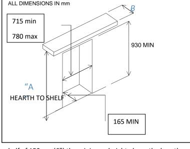
minimum clearance above the appliance of 200mm. For a shelf of 150mm (6") the minimum height above the hearth or base of opening must be 1045mm. This will give a minimum clearance above the appliance of 300mm.
